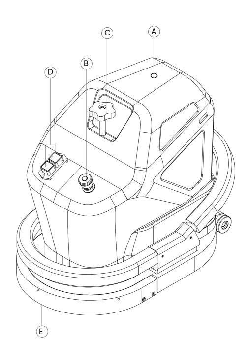
**A- Electrical cable.** the 48 volt current has to travel 6 metres long; the cable must always be connected to the central conversion unit by a special plug.
